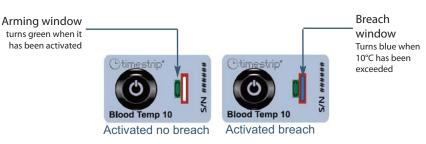
If the temperature increases above 10°C during transport or storage phases of the blood bag, the breach window is changed from white to blue, indicating that the blood has been contaminated.
