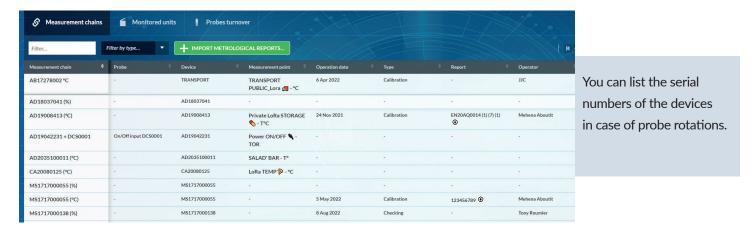
Calibration results and threshold corrections are automatically taken into account in the JRI-MySirius software.
